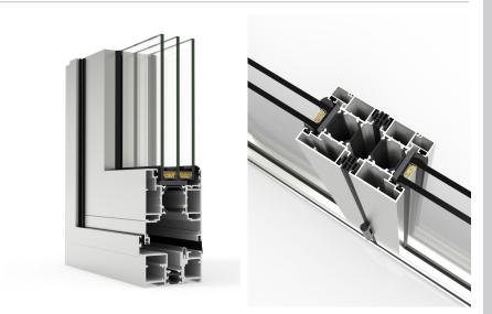
Thermally broken system with 73 mm of frame depth, ideal to divide environments and unify spaces both in residential and commercial buildings. It allows multiple combinations of up to 14 sashes that allow to close spans of more than 16 meters wide. It has slim sightlines and hidden rollers, showing a clean aesthetic in the closed position. In addition, the flush threshold facilitates accessibility and transit between the interior and exterior.
